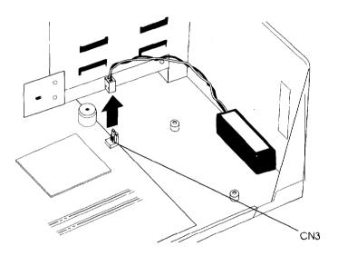
3. The battery is attached to the computer base with Velcro. To remove it, pull it up from the bottom of the computer case, as shown in the following illustration. Then set it aside.
